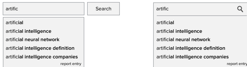
Fig. 1. The figure shows the wireframes of textual autocompletion in the special case of query autocompletion. Both versions offer the same functionality. They make partial user input more complete. On the left: A user interface composed of three components, an input field, a suggestion area, and a button for confirmation. With loose interface elements. On the right: A more compact version with adapted visual composition. The search button was replaced by an icon of a magnifying glass. The search field and the suggestion area are combined into one field. Both examples show an option in the bottom right of the suggestion area to report inappropriate entries.
